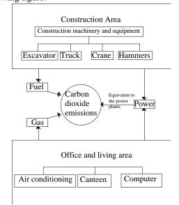
As is shown in the figure, by summarize the carbon emissions from the construction phase, we can see that it is made primarily of fossil energy consumption and energy consumption of the composition. So energy consumption will produce carbon dioxide, which mainly include energy consumption the use of mechanical equipment secondary transport in construction site, as well as the transportation of building garbage and building materials.
